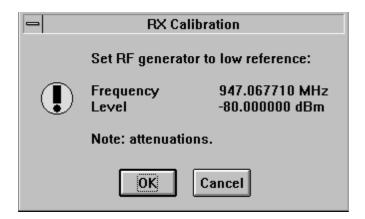
4. Measurement with low input level is executed
